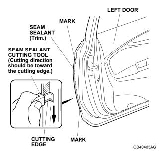
6. Apply touch-up paint to the cut seam sealant area, and let it to dry thoroughly.
